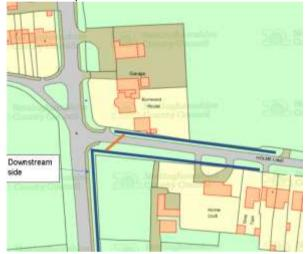
Ditches are in blue, the highway culvert in orange. The outlet of the highway culvert is partially collapsed. It's directly adjacent to a large tree and there is a possibility that it may have been damaged by roots from the tree. I'll get a job raised for my colleagues in the Drainage Maintenance team to attend to jet and cctv the culvert. I can't give you a timescale for this at present, but it will hopefully be sometime next month.
