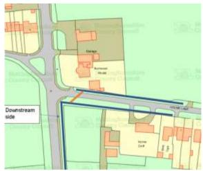
Ditches are in blue, the highway culvert in orange. The outlet of the highway culvert is partially collapsed. It's directly adjacent to a large tree and there is a possibility that it may have been damaged by roots from the tree. I'll get a job raised for my colleagues in the Drainage Maintenance team to attend to jet and cctv the culvert. I can't give you a timescale for this at present, but it will hopefully be sometime next month.
