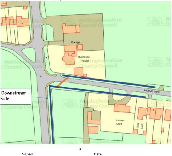
Ditches are in blue, the highway culvert in orange. The outlet of the highway culvert is partially collapsed. It's directly adjacent to a large tree and there is a possibility that it may have been damaged by roots from the tree. I'll get a job raised for my colleagues in the Drainage Maintenance team to attend to jet and cctv the culvert. I can't give you a timescale for this at present, but it will hopefully be sometime next month.
